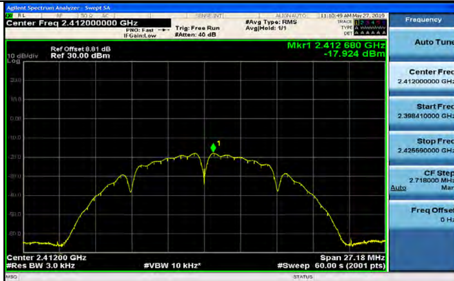
Maximum(average) power spectral density_11B_2437_Ant1
