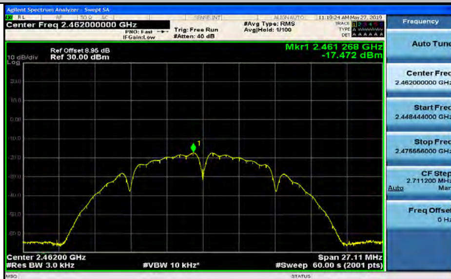
Maximum(average) power spectral density_11B_2462_Ant1
