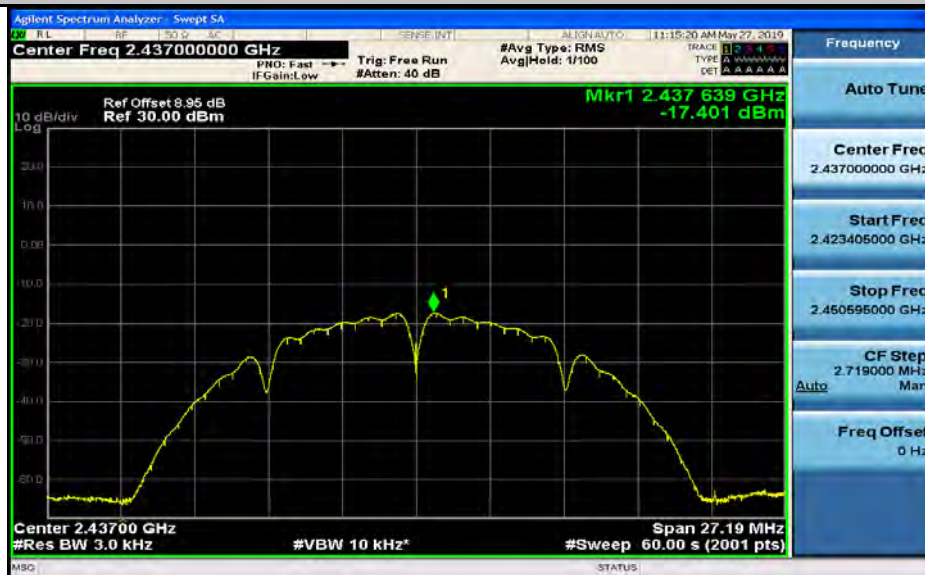
Maximum(average) power spectral density_11B_2462_Ant1
