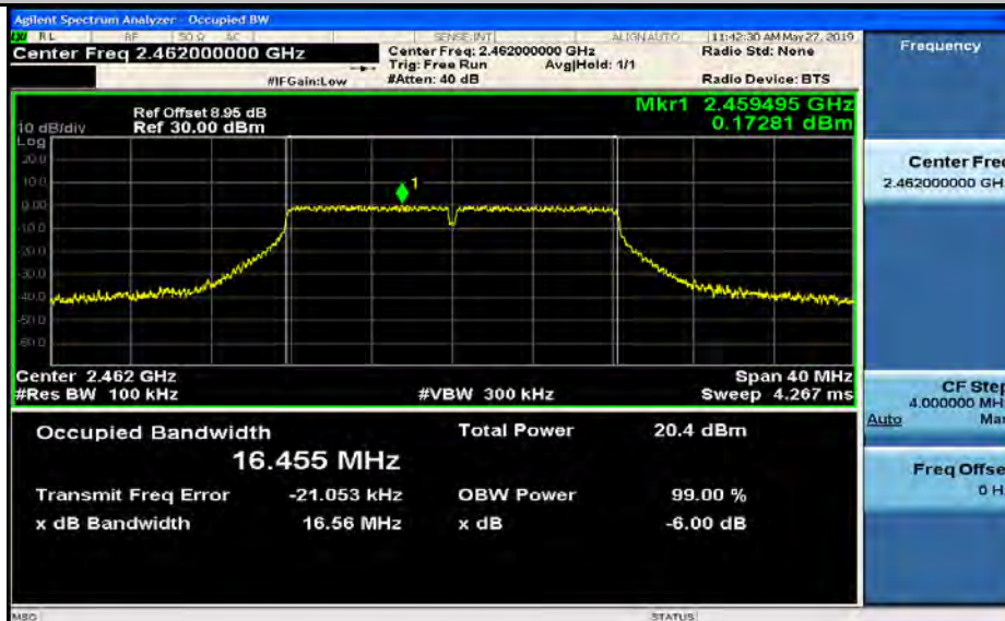
6dB Bandwidth_11N20SISO_2462_Ant1
