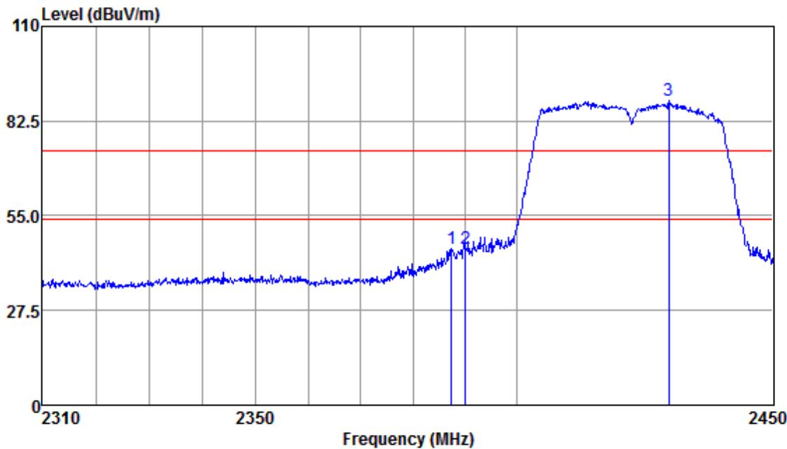
Mode:a; Polarization:Vertical; Modulation:n; bandwidth:40MHz; Channel:Low
