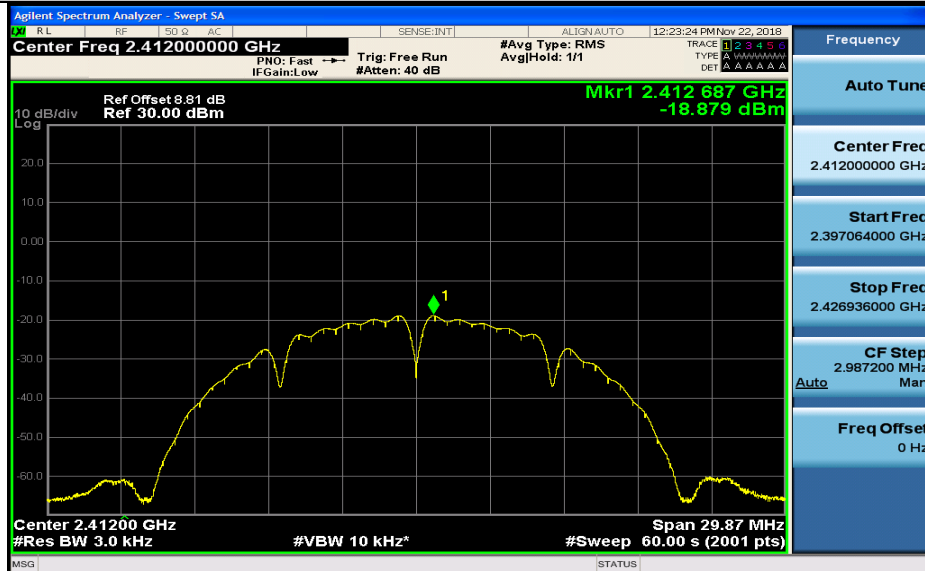
Maximum(average) power spectral density_11B_2437_Ant1
