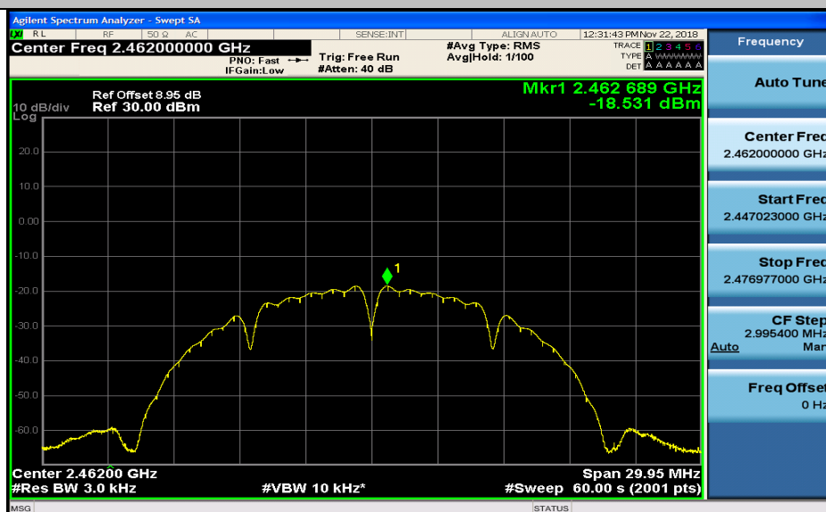
Maximum(average) power spectral density_11B_2462_Ant1
