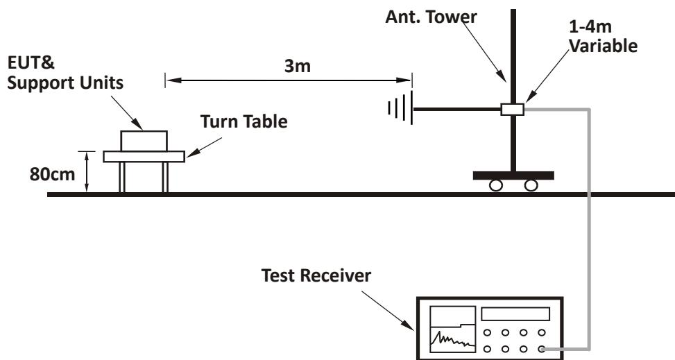
**TEST REPORT****For Radiated emission above 1GHz:**
