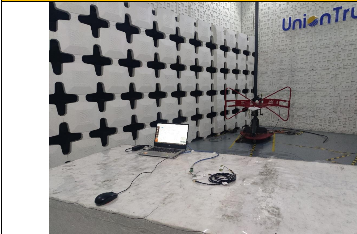
Radiated emission Test Setup (30 MHz~1 GHz)
