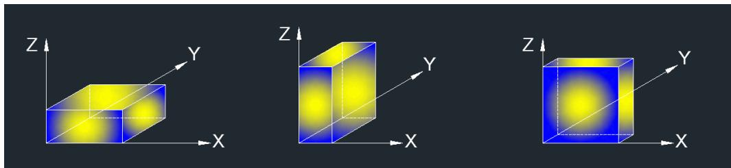
Note: For all radiated test, EUT had been tested in X axis position according to the user manual that the product should be installed in X axis position.
