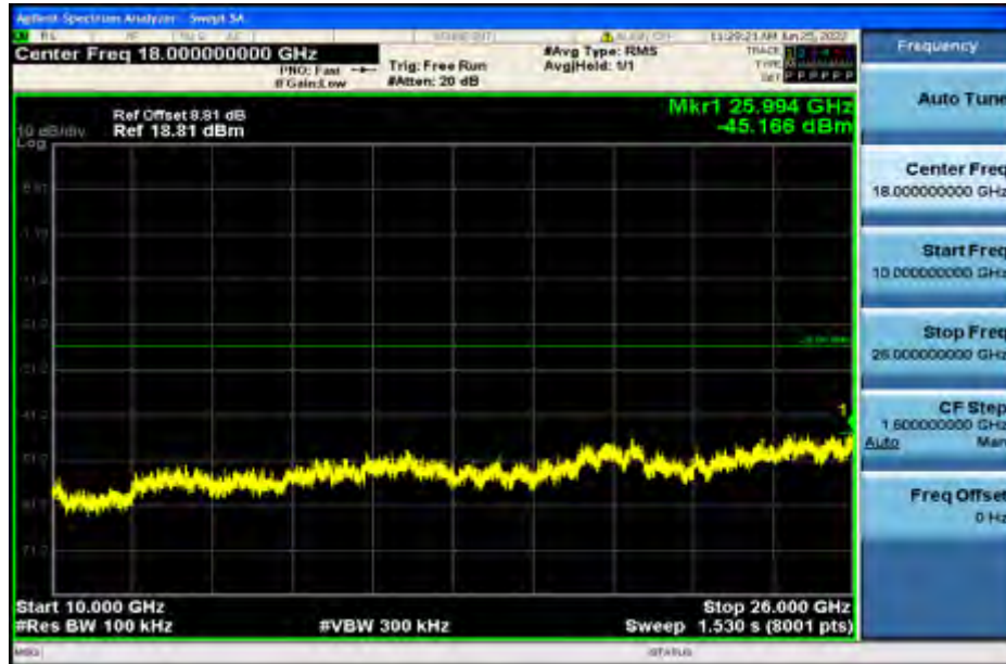
RF Conducted Spurious Emissions_11B_2437
