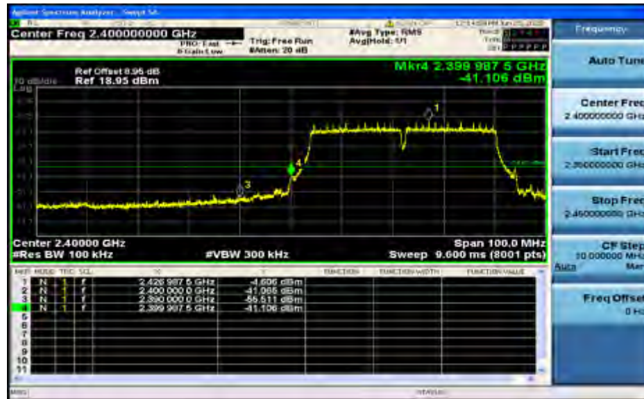
Band-edge for RF Conducted Emissions_11N40SISO_2452_Ant1
