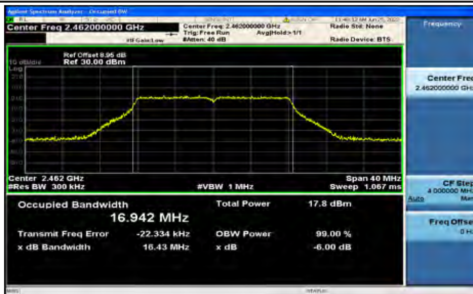
Occupied Bandwidth_11N20SISO_2412
