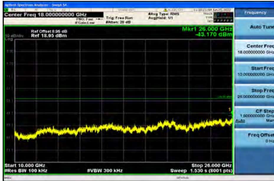
RF Conducted Spurious Emissions_11G_2412
