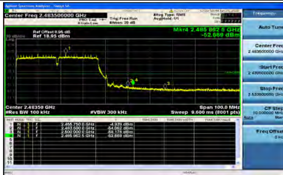
Band-edge for RF Conducted Emissions_11N40SISO_2452_Ant1
