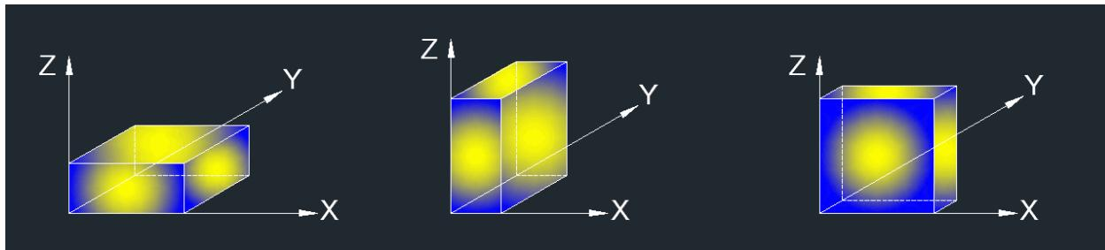
Note: For all radiated test, EUT in each of three orthogonal axis emissions had been tested, but only the worst case (X axis) data recorded in the report.
