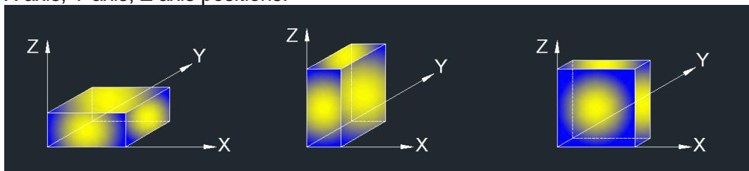
Note: For all radiated test, EUT in each of three orthogonal axis emissions had been tested, but only the worse case (X axis) data recorded in the report.
