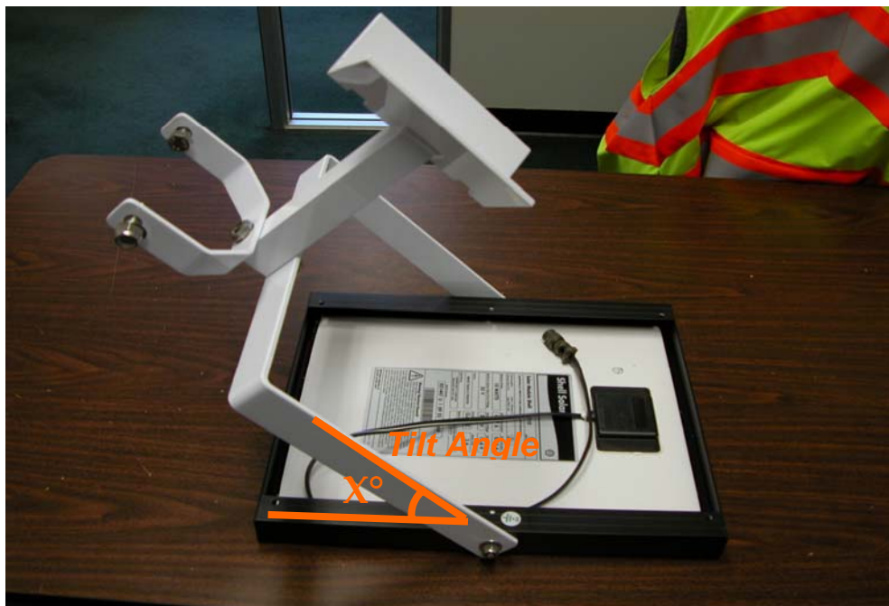
Figure 3 - Sensor Sub-assembly showing solar panel tilt angle
