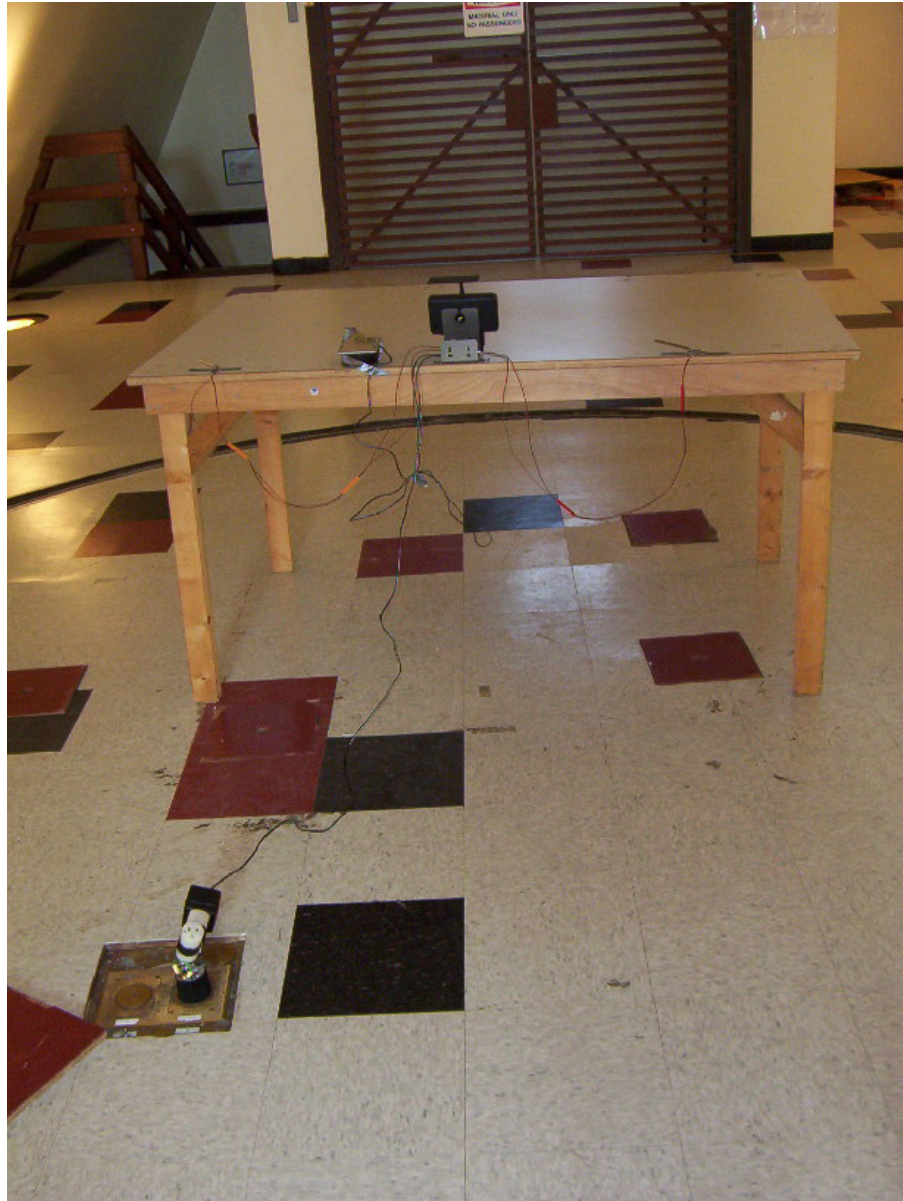
Radiated Emission Test Setup – Rear View
