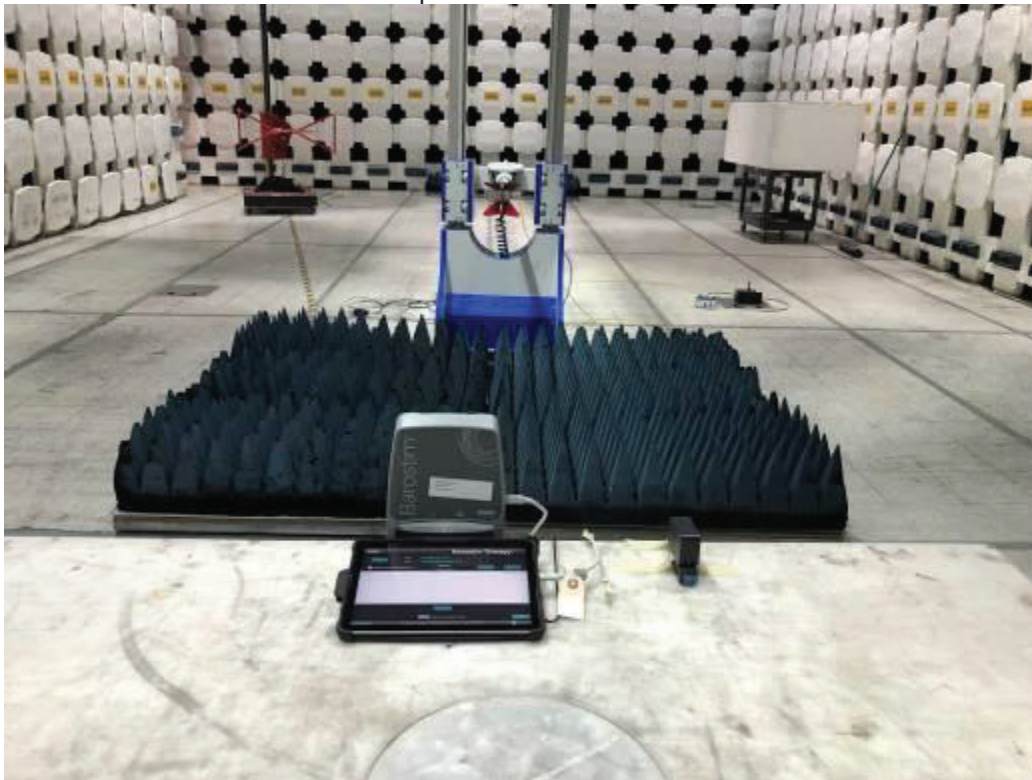
Test Setup Above 1 GHz at 3 meters
