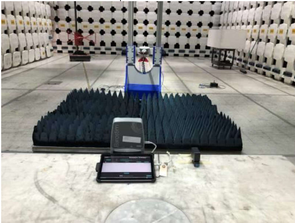
Test Setup Above 1 GHz at 3 meters
