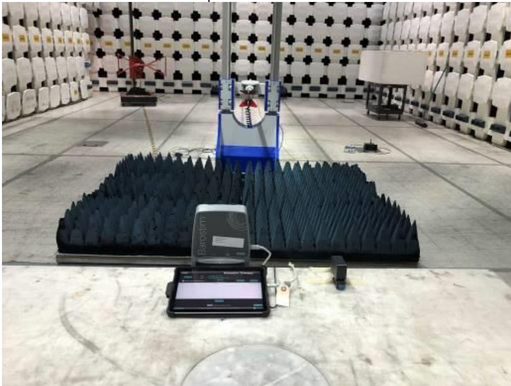
Test Setup Above 1 GHz at 3 meters
