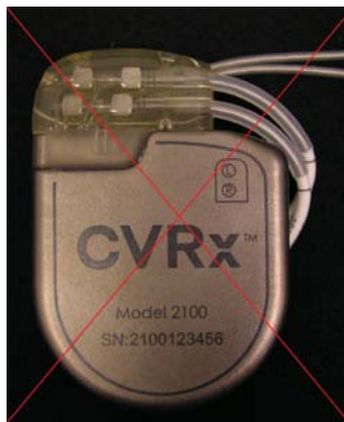
Incorrect placement of lead behind IPG
