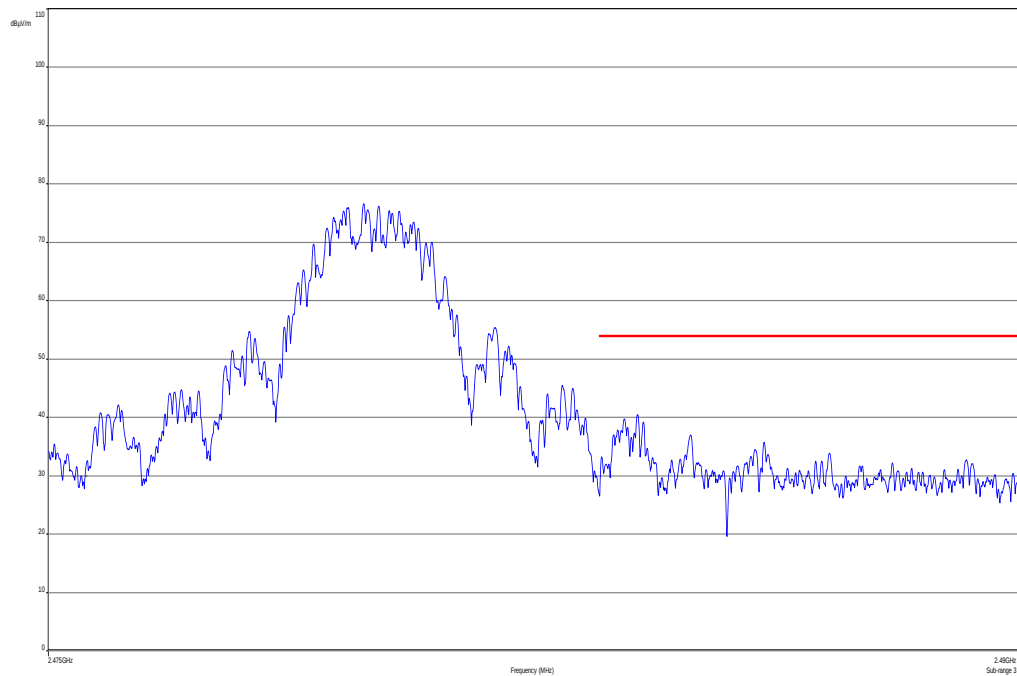
Plot 3: additional channel, 2480 MHz, upper band edge, vertical & horizontal polarization
