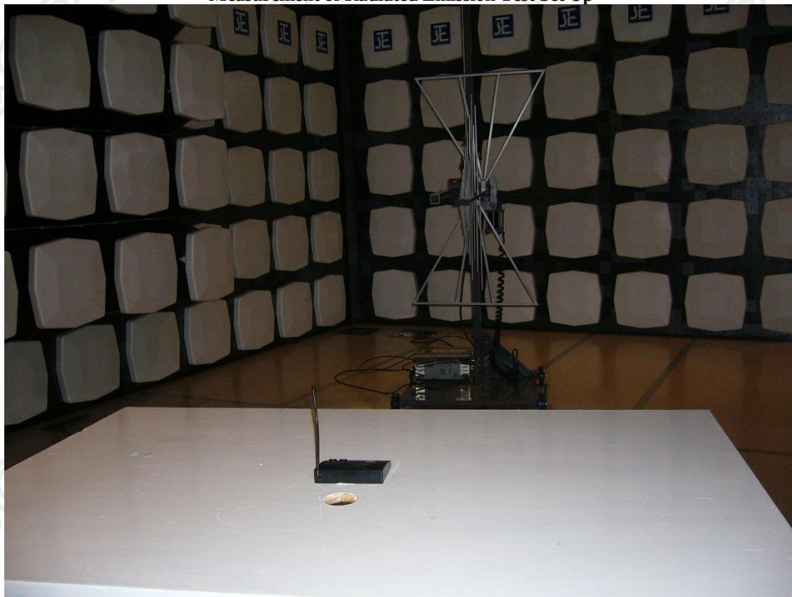
Measurement of Radiated Emission Test Set Up
