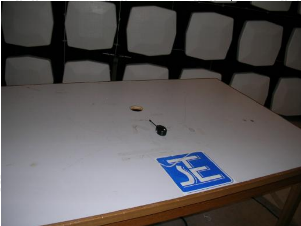
Measurement of Radiated Emission Test Set Up
