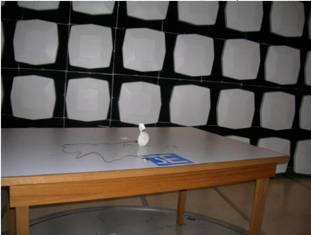
Measurement of Radiated Emission Test Set Up
