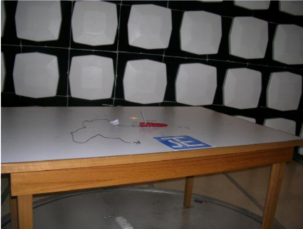
Measurement of Radiated Emission Test Set Up
