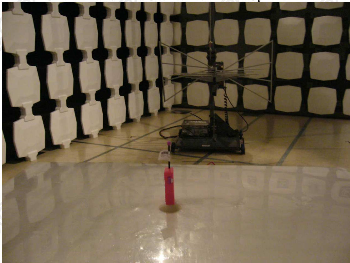
Measurement of Radiated Emission Test Set Up
