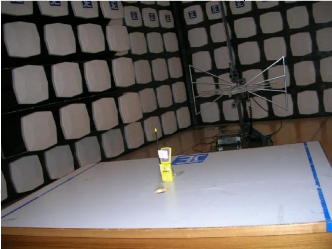
Measurement of Radiated Emission Test Set Up
