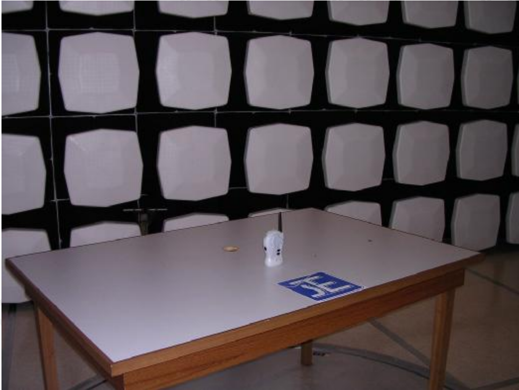
Measurement of Radiated Emission Test Set Up
