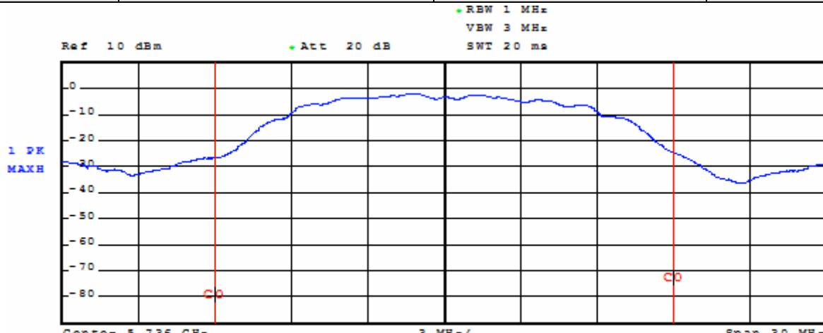
Tx Channel Bandwidth 18 MHz Power 6.24 dBm
