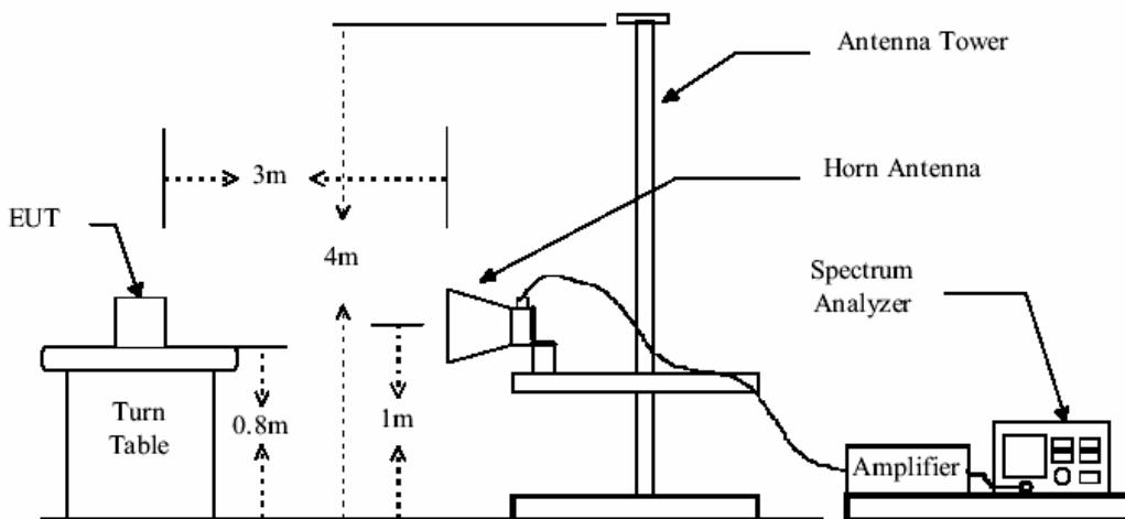
Low noise amplifier was used below 1GHz, High pass Filter was used above 1GHz.
