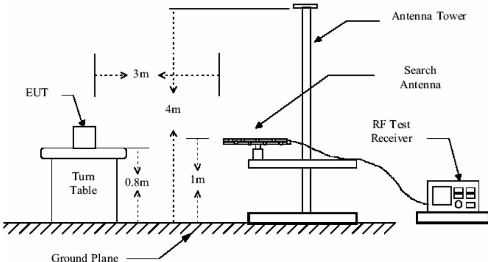
Radiated Emission Test Set-up Frequency Over 1GHz
