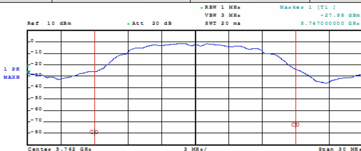
Tx Channel Bandwidth 18 MHz Power 7.06 dBm
