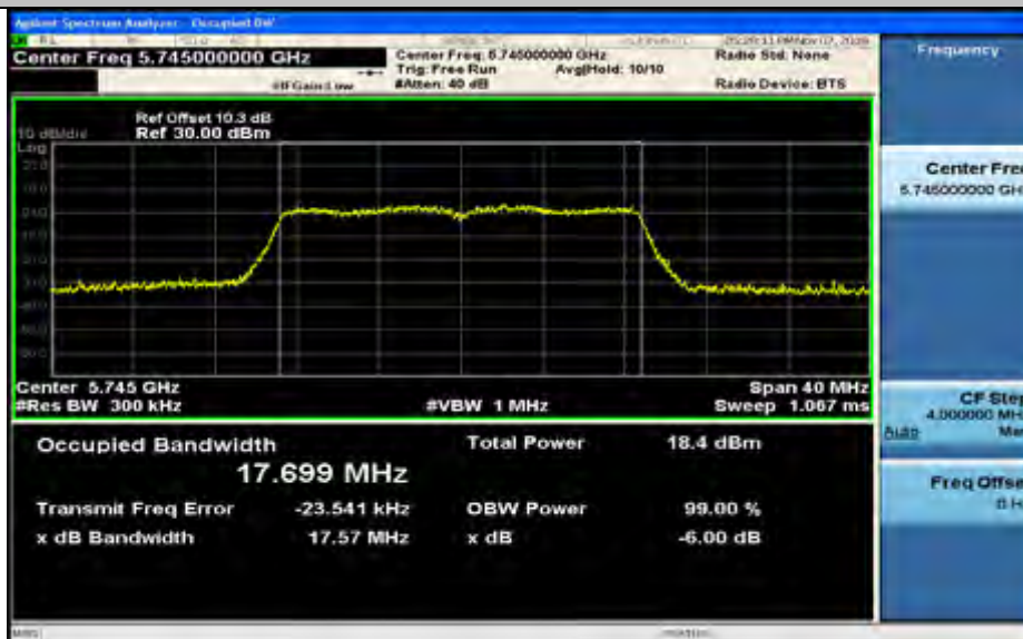
Occupied Bandwidth Measurement_11N20_5785_Ant1
