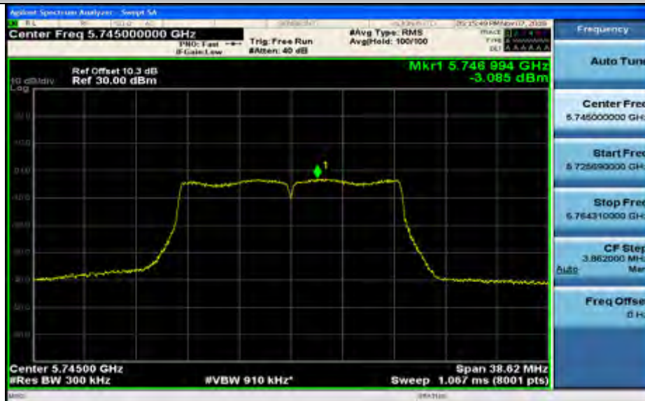
Maximum Power Spectral Density_TNVN_11A_5785_Ant1
