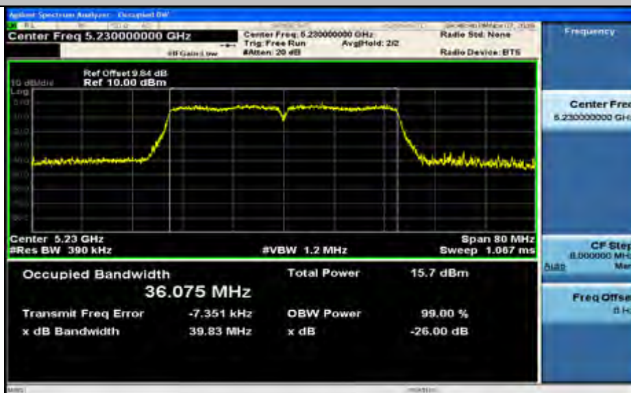
(26dB)Emission Bandwidth Measurement_11AC40_5230_Ant1
