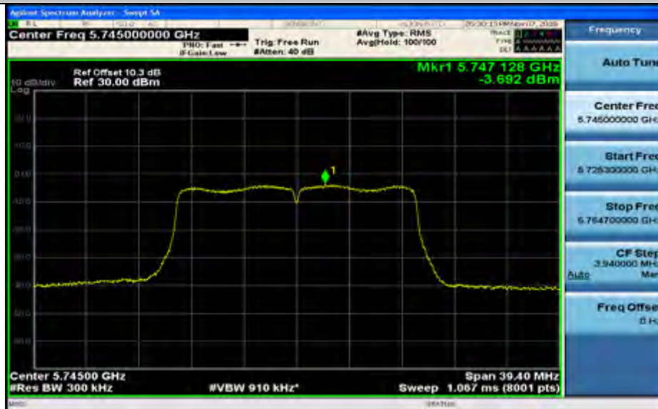
Maximum Power Spectral Density_TNVN_11N20_5785_Ant1
