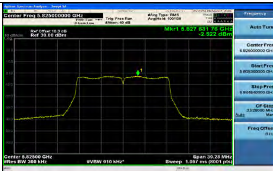
Maximum Power Spectral Density_TNVN_11N20_5180_Ant1
