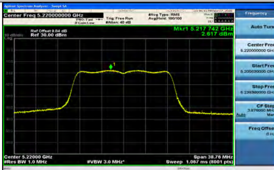
Maximum Power Spectral Density_TNVN_11A_5240_Ant1
