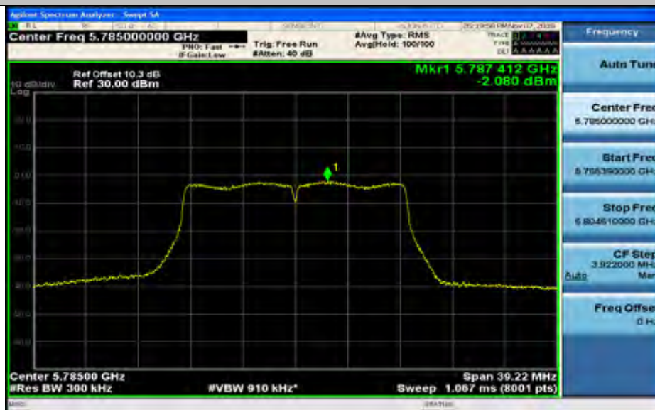
Maximum Power Spectral Density_TNVN_11A_5825_Ant1
