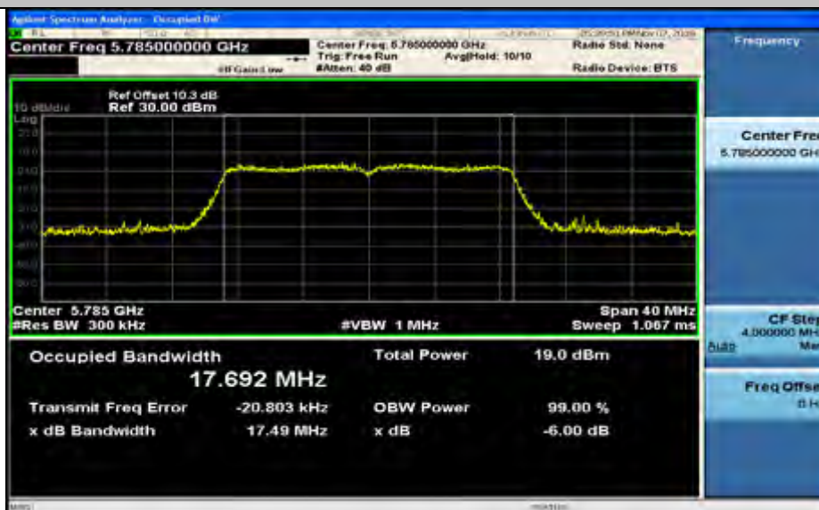
Occupied Bandwidth Measurement_11N20_5825_Ant1
