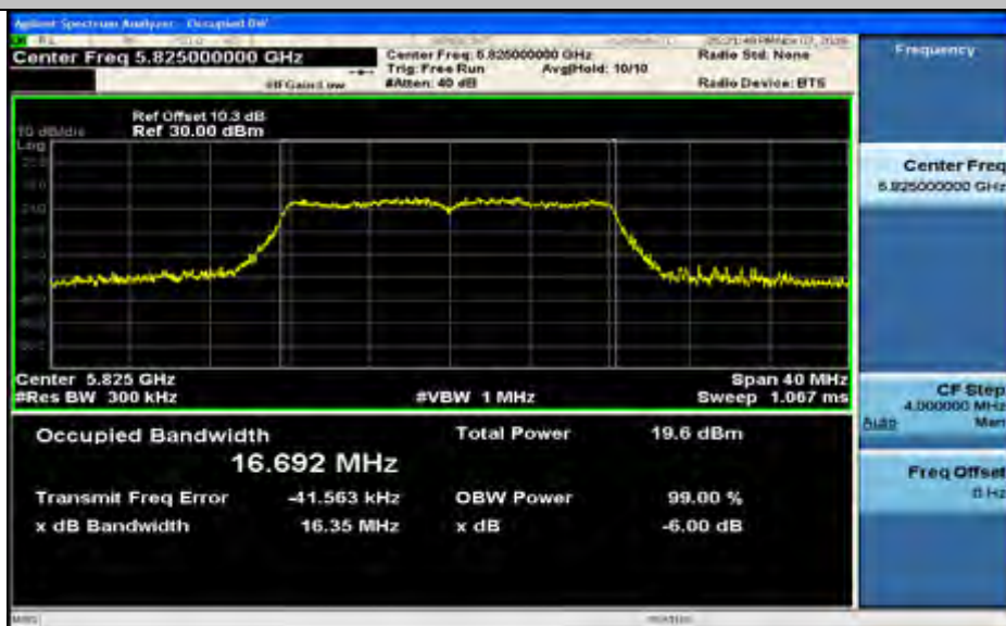
Occupied Bandwidth Measurement_11A_5825_Ant1
