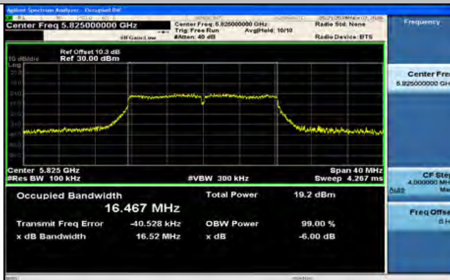
(6dB)Minimum Emission Bandwidth Measurement_11A_5825_Ant1
