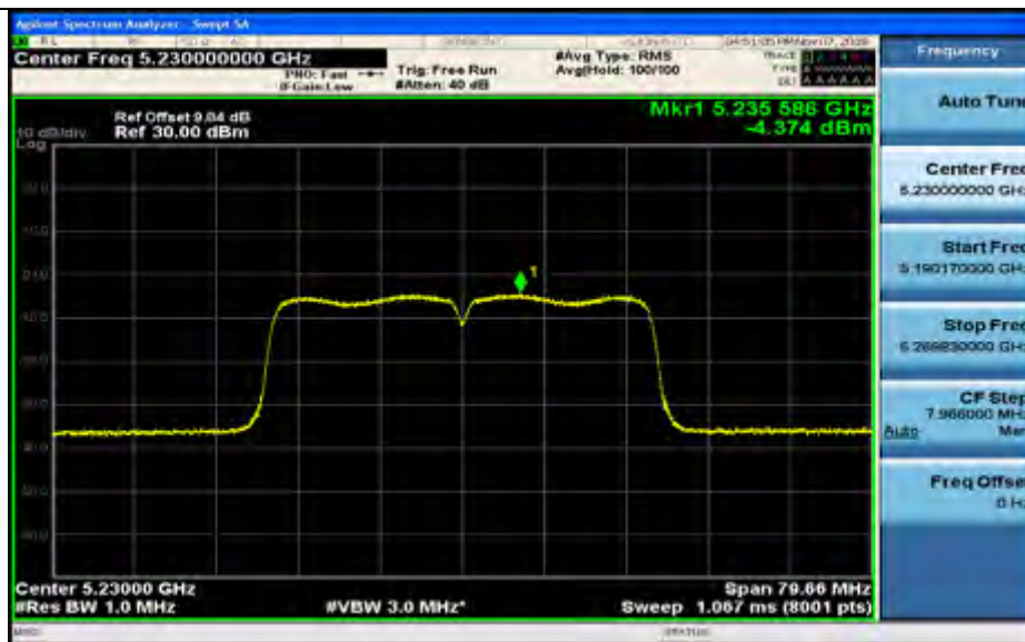
Maximum Power Spectral Density_TNVN_11AC40_5755_Ant1
