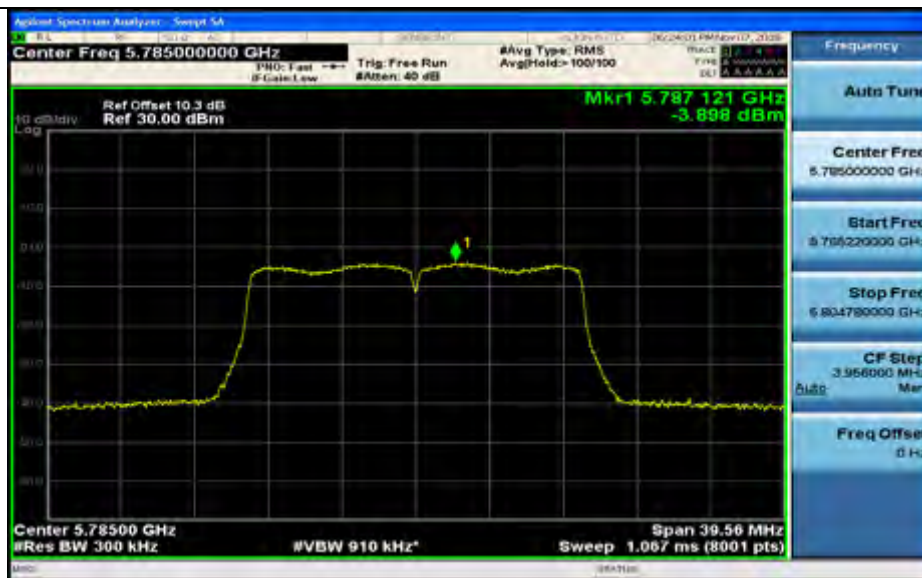
Maximum Power Spectral Density_TNVN_11AC20_5825_Ant1
