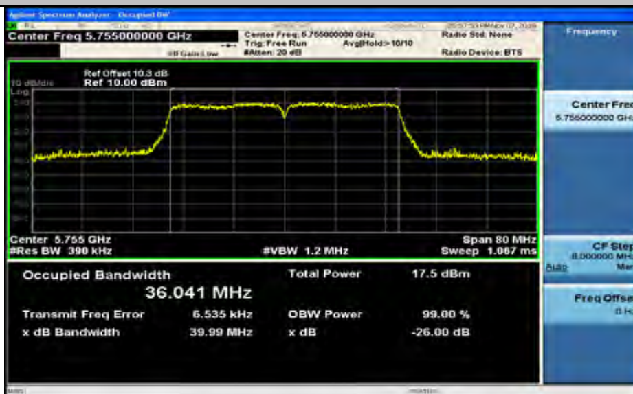
(26dB)Emission Bandwidth Measurement_11N40_5755_Ant1
