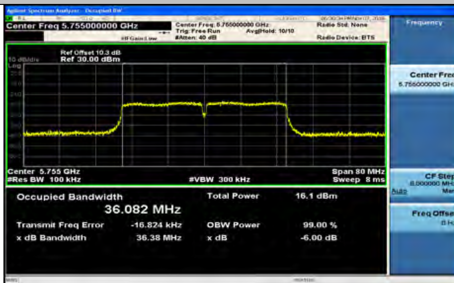
(6dB)Minimum Emission Bandwidth Measurement_11AC40_5755_Ant1
