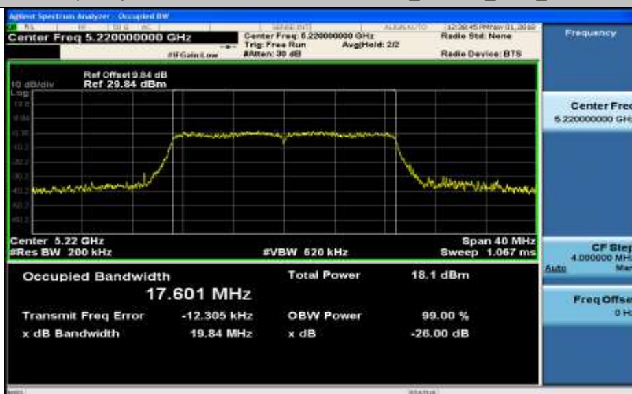
(26dB)Emission Bandwidth Measurement_11AC20_5220_Ant1
