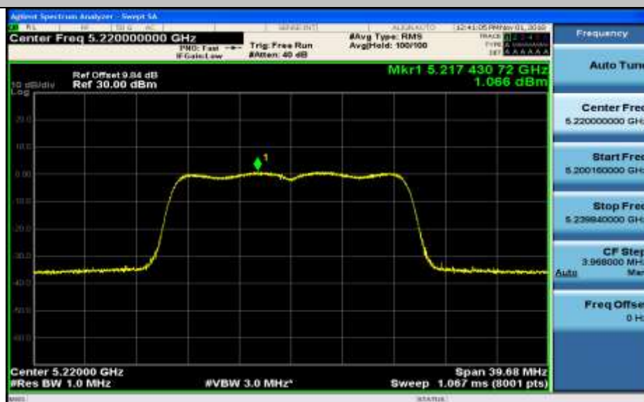
Maximum Power Spectral Density_TNVN_11AC20_5220_Ant1
