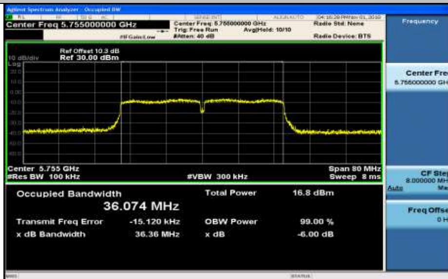
(6dB)Minimum Emission Bandwidth Measurement_11AC40_5755_Ant1
