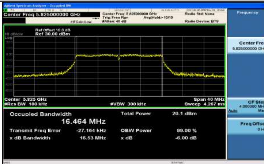
(6dB)Minimum Emission Bandwidth Measurement_11A_5825_Ant1
