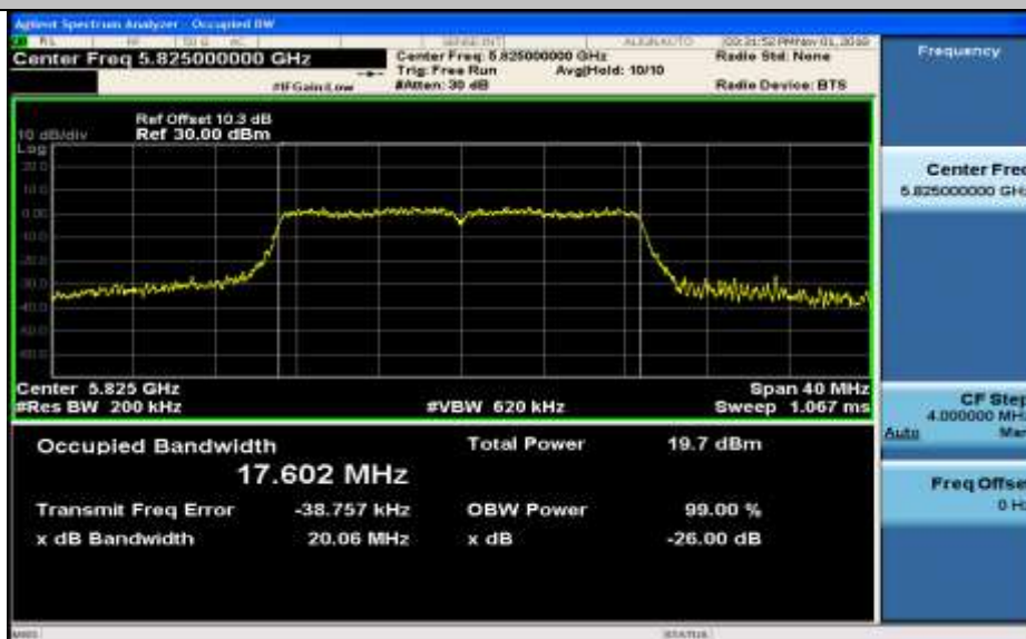
(26dB)Emission Bandwidth Measurement_11N20_5825_Ant1
