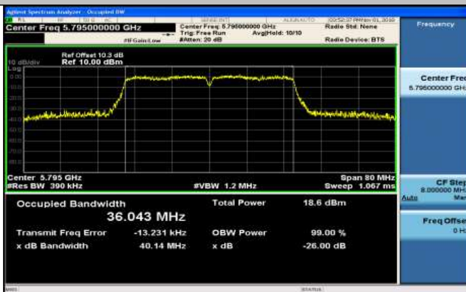
(26dB)Emission Bandwidth Measurement_11AC20_5180_Ant1
