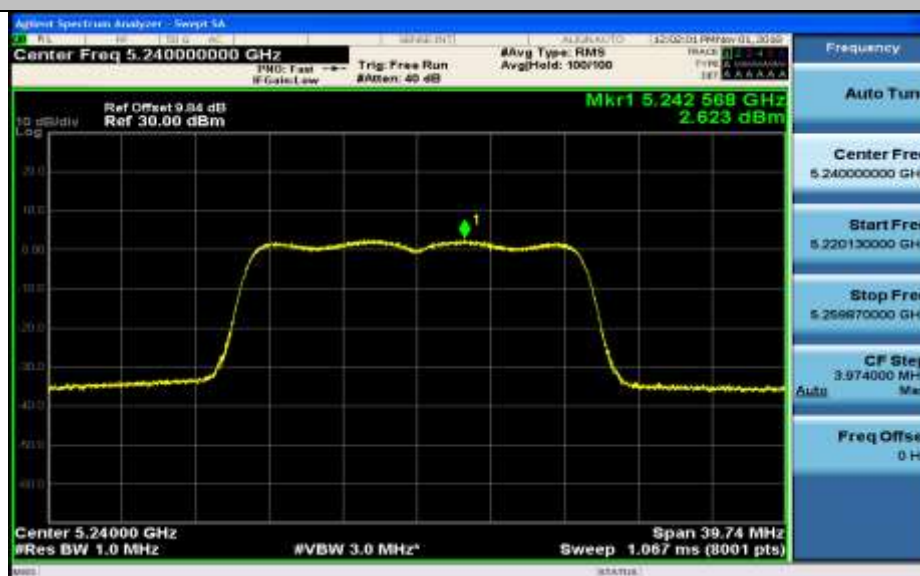
Maximum Power Spectral Density_TNVN_11N20_5240_Ant1
