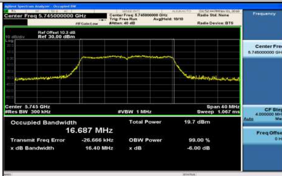
Occupied Bandwidth Measurement_11A_5785_Ant1
