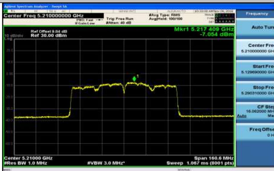
Maximum Power Spectral Density_TNVN_11AC80_5210_Ant1
