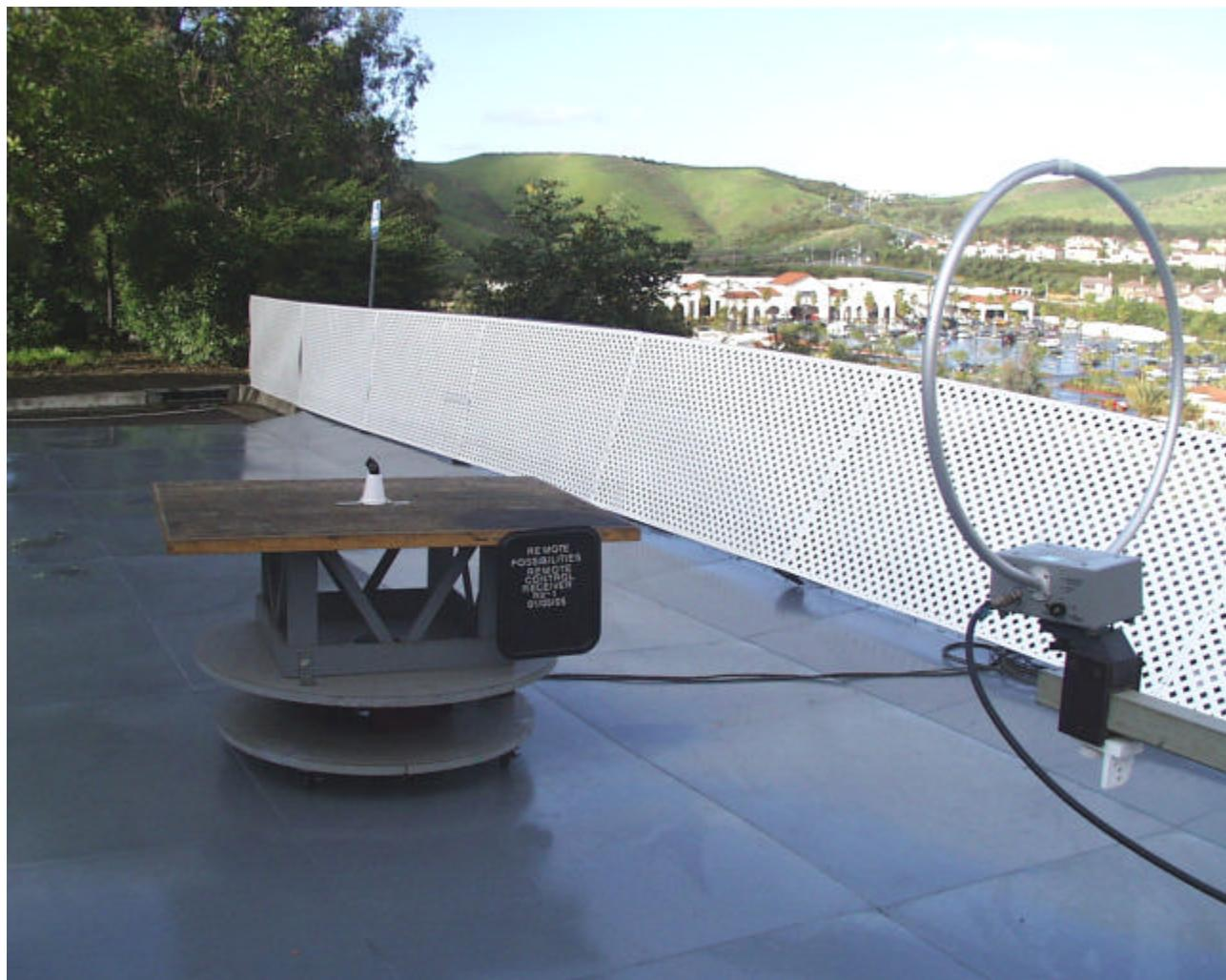
**Radiated Emissions with Active Loop Antenna**
