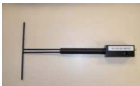
Figure 1 – Satimo COMOSAR Validation Dipole
