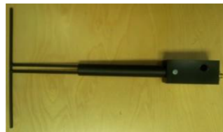
Figure 1 – MVG COMOSAR Validation Dipole
