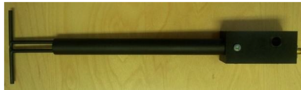
Figure 1 – MVG COMOSAR Validation Dipole
