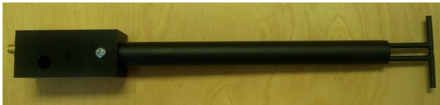
Figure 1 – MVG COMOSAR Validation Dipole
