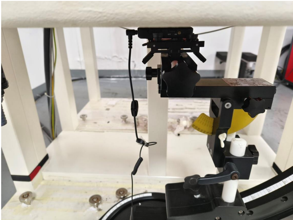
The thickness of EUT is 17mm Limbs Front with headset 0mm
