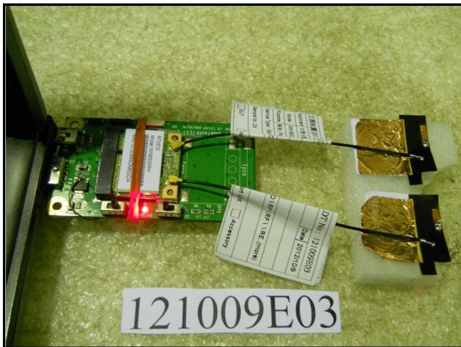
RADIATED EMISSION TEST (WLAN 5GHz Band) **(PIFA Antenna)**
