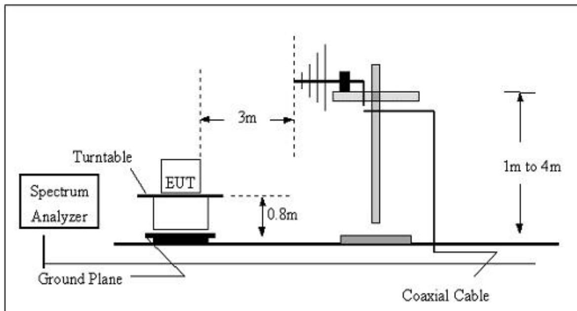
**Radiated Emission Test Set-Up, Frequency Over 1GHz**
