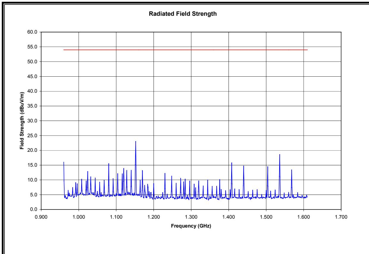
**FIELD STRENGTH 0.960 TO 1.610 GHz, 1 MHz BW, HORIZONTAL, PEAK**
