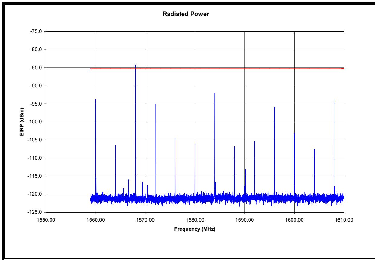
Note: All emissions above the limit line were identified as unintentional digital device emissions. None of the emissions above the limit line are due to the UWB radio.
