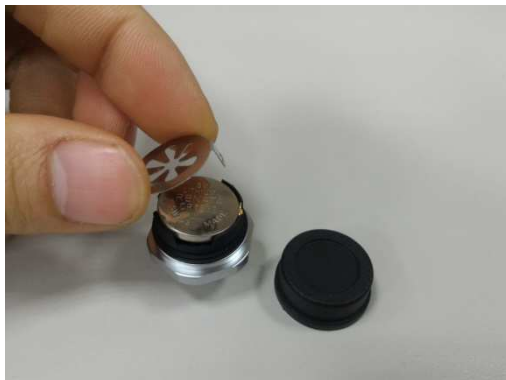
Install battery into sensor
