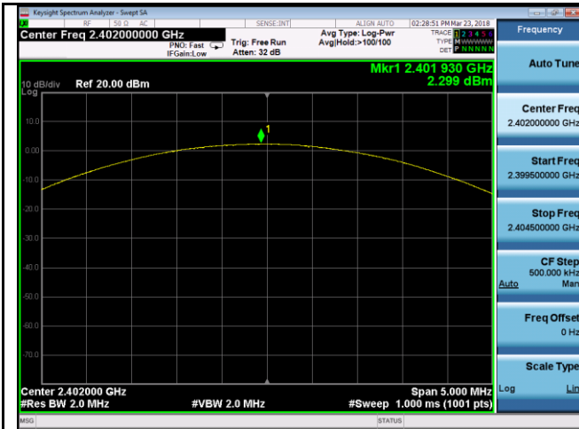
8DPSK Output power - Low CH 2402
