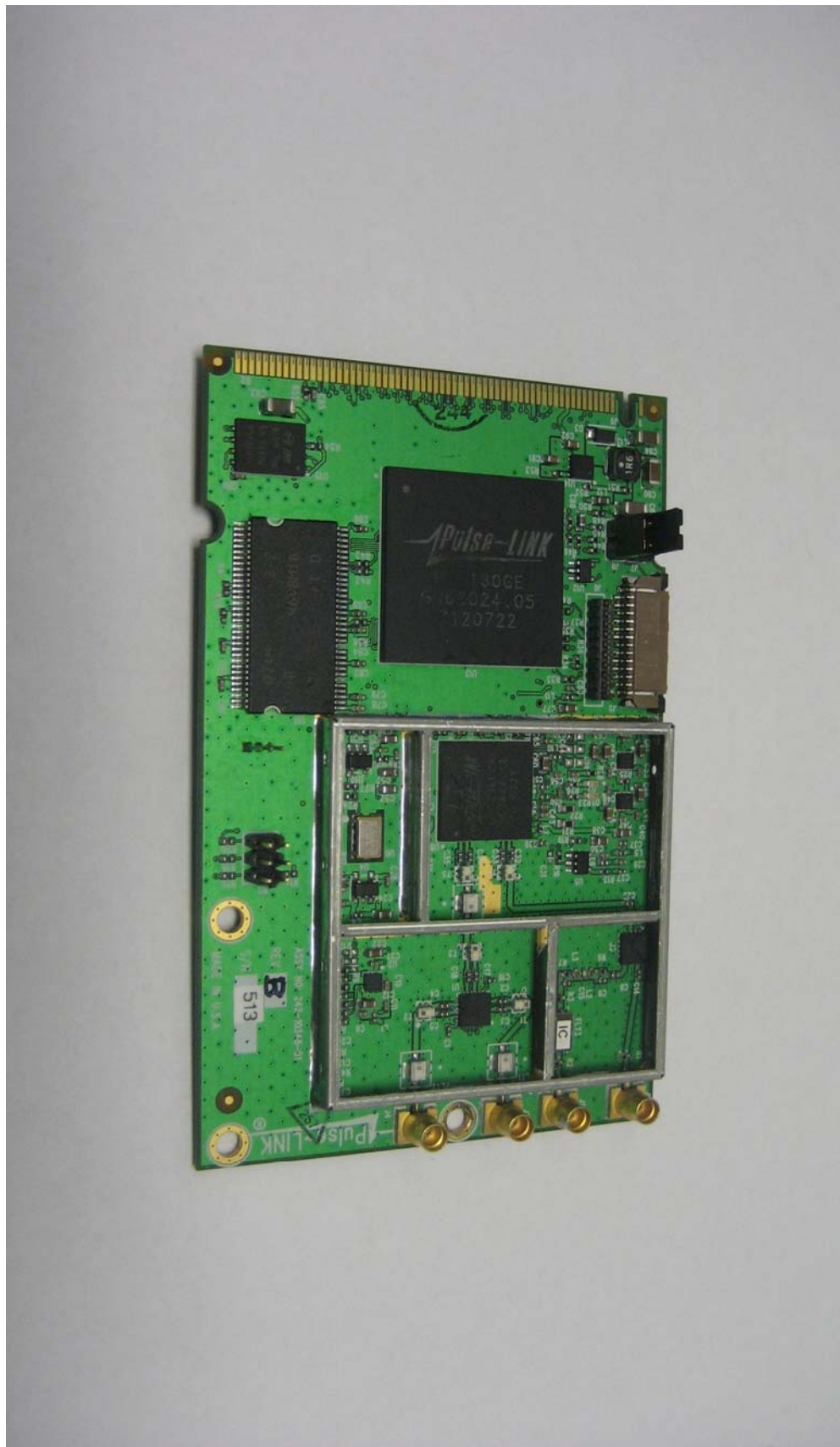
Figure 3. Top side of PL3301 with shield removed.
