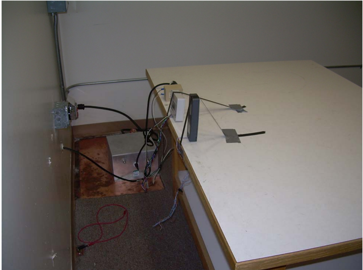
Back View Conducted Disturbance Worst Case Configuration
