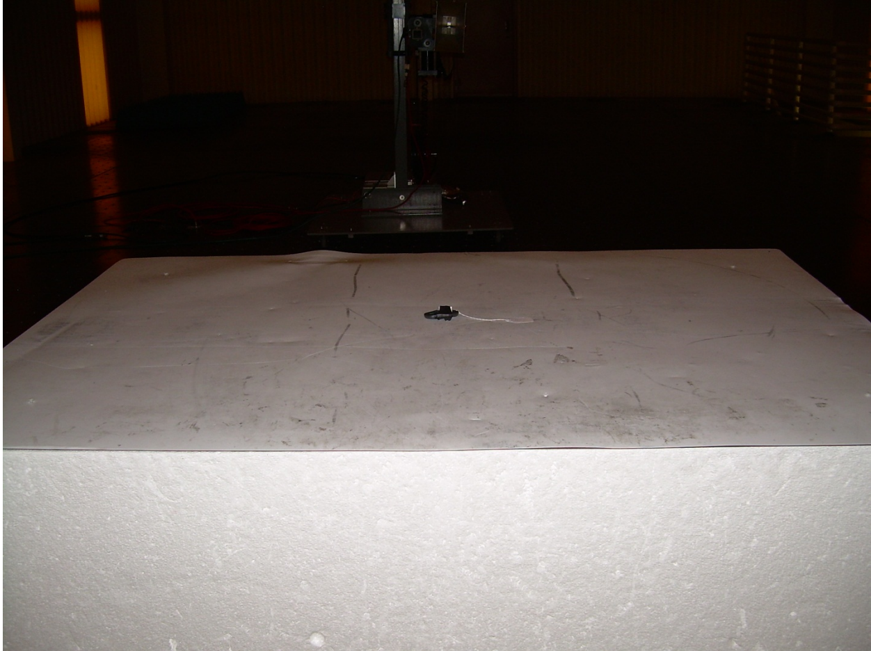
Photograph 1 – View Radiated Emission Configuration – Horizontal Orientation
