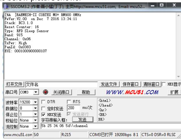
3. Provide a Host installed a same modem working on Coordinator mode, host's modem info is showing as below picture. They are at the same band 915.
