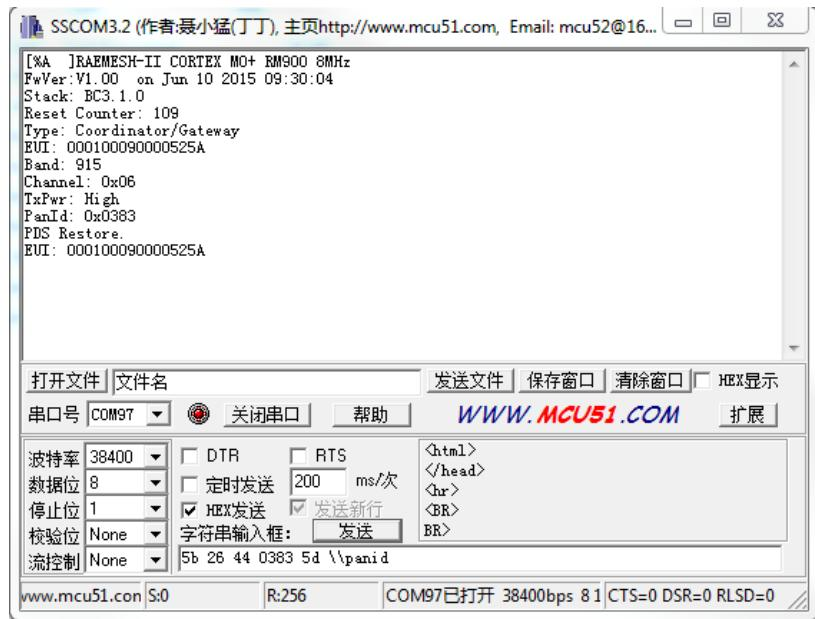
4. Send command “5b 25 34 01 5d” to set host and end modem to same channel, HEX “01” means channel 1 (906MHz), HEX “0A” means channel 10 (924MHz);
