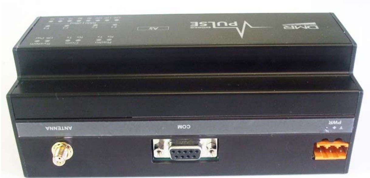
External Views: Face showing connectors
