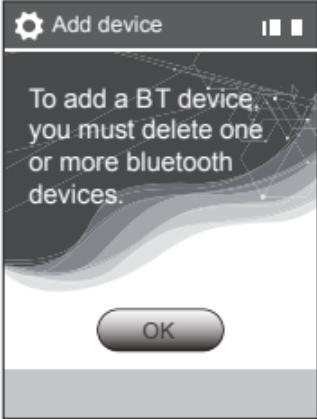
A screenshot of a mobile device's screen titled "Add device". The main message says "To add a BT device, you must delete one or more bluetooth devices." with a small graphic of a network or waves below it. At the bottom is a grey "OK" button. | <p>※ The maximum number of Bluetooth devices registered is 8.</p>                                                                                                                                            |
