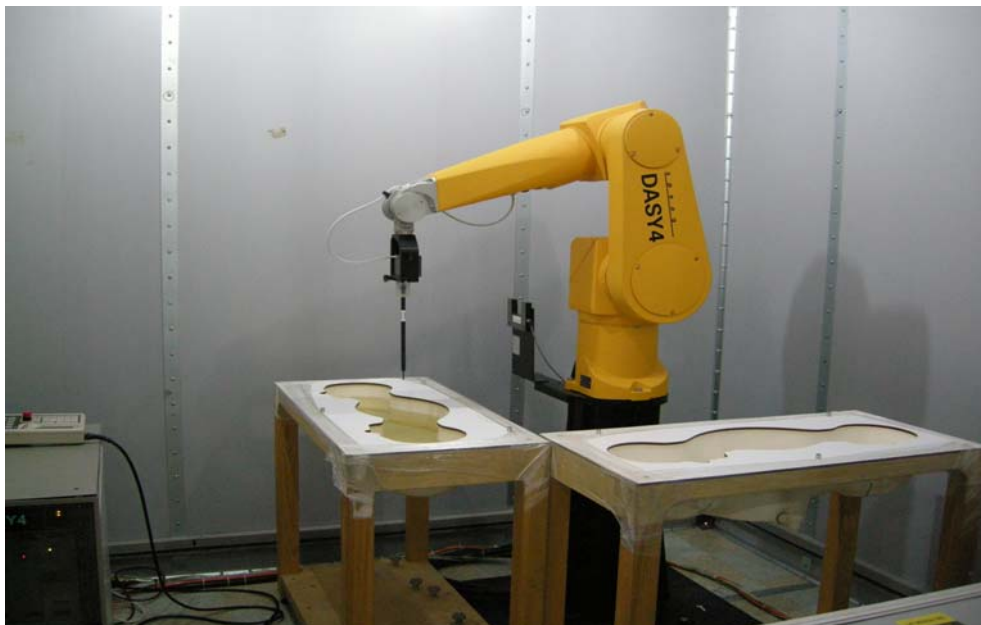
Fig. 4.1 SAR Measurement System
