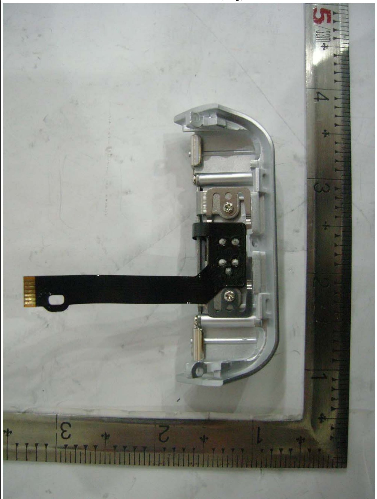
View of Sub 4 PCB(Top)
