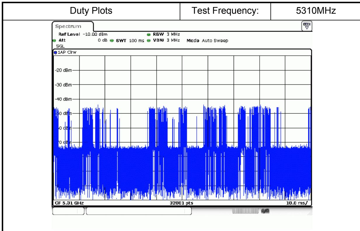
**Test Result of Channel Shutdown Time Plots**
