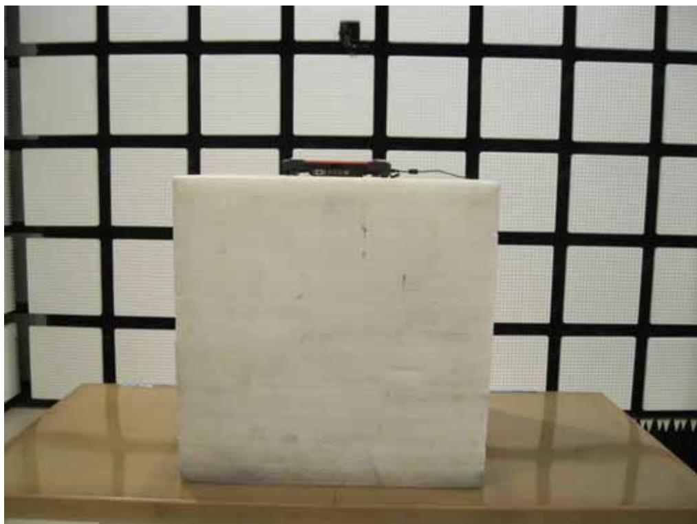
**ANTENNA PORT CONDUCTED RF MEASUREMENT SETUP**
