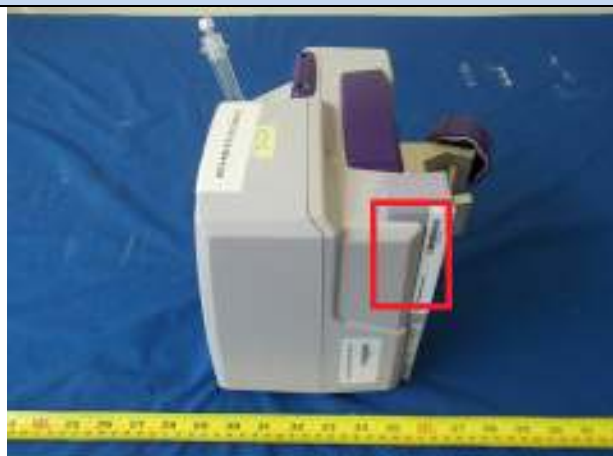
Right edge position against flat phantom (Ant #1 & #2 location) (separation distance – 0cm)
