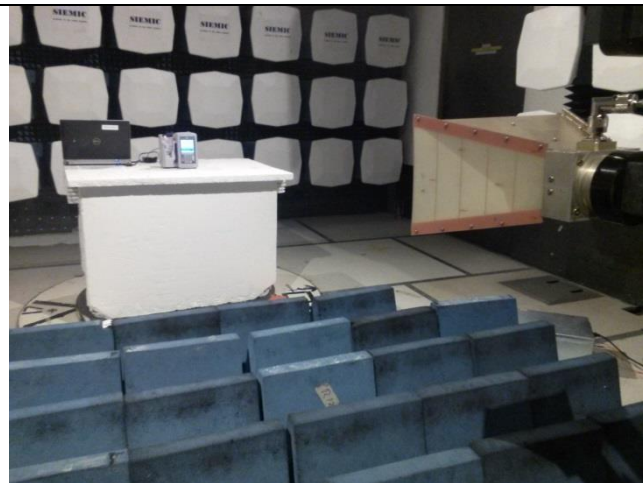
Test setup at 3 meter distance (>1GHz) - Front
