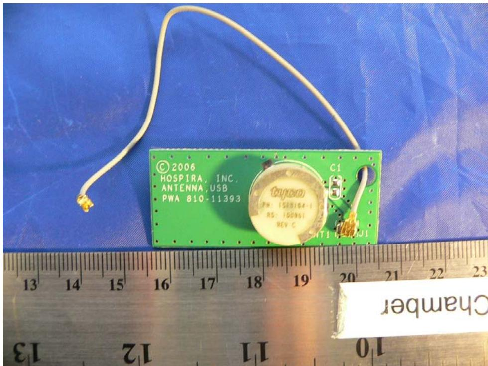
**EUT – PCB Antenna Solder Side View**
