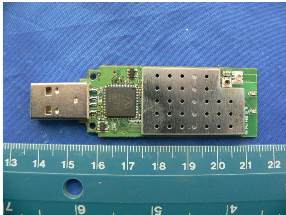
**EUT (Model: 20677-04-XX) – Wireless USB Dongle Component Side View (RF shielding removed)**
