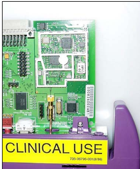
RF board with Cans removed
