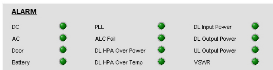
Figure 5.14 ALARM Indication Window
